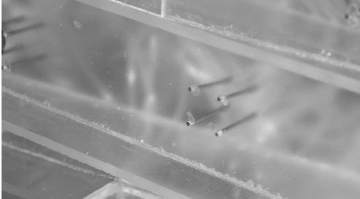
Figure 2.7: Photo of a pressure tap cluster on model. Each pressure tap has a full-scale equivalent area of less than 1 \text{ m}^2 .
