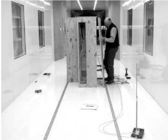
Figure 2.11: 1:25 scale model of two skin façade of a block building in Søndermarken in Copenhagen. The photo shows the model in the large wind tunnel of SOH Wind Engineering in Vermont, USA. The vertical oriented cavity is shown in the middle of the photo, where the model is constructed of plexiglass. Reproduced by permission of Moe, Consulting Engineers, and the building owners, KAB.
